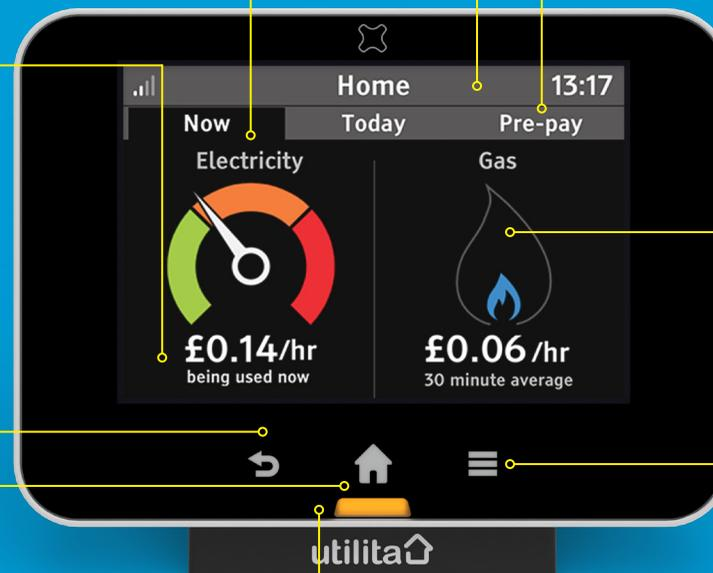
The banner bar allows you to check the smart meter(s) signal strength and time.
